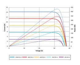
Current-Voltage & Power-Voltage Curve (4305)
